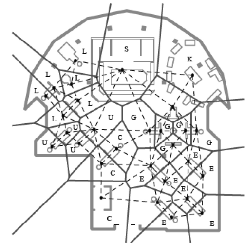
(3d) Great Lakes Science Center, ZAP Voronoi Regions Delaunay Triangulation 1m 5m 10m
